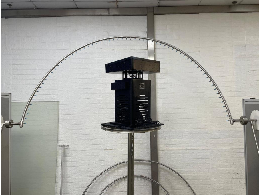
Photo 3: IPX4 test of model H-BS700-TYN
