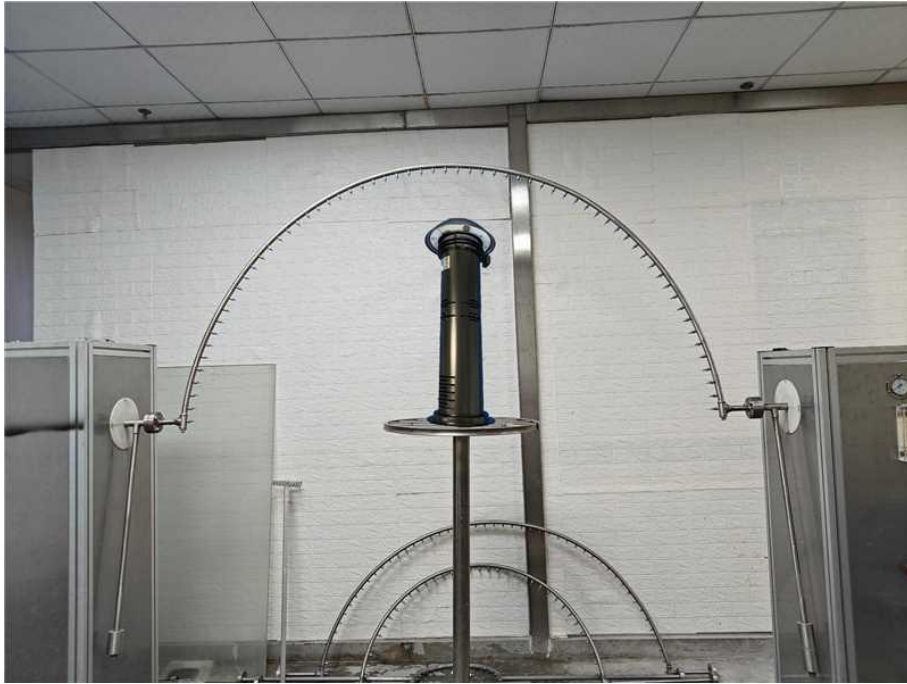
Photo 3: IPX4 test of model H-X5(APP)
