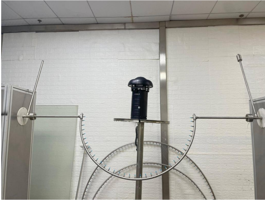
Photo 3: IPX4 test of model H-X3(APP)
